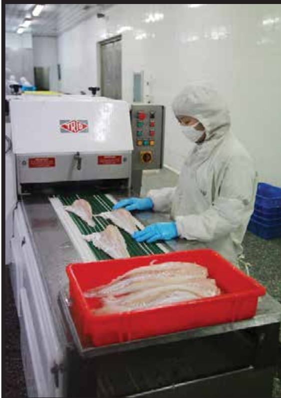
Cod Fillets being deep-skinned on Trio Skinning Machine
